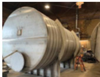
Precision Tank (PT), part of Precision Build Companies, recently completed fabrication and delivery of three 11' diameter x 21' tall stainless-steel shop-built tanks. These tanks were built at the PB facility in Virginia, Illinois.
