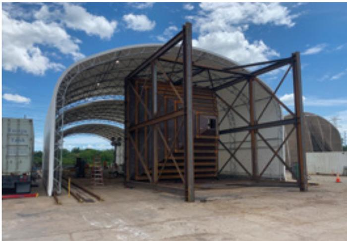
PB recently fabricated and shipped three hoppers that are to be used for unloading aggregate from ocean vessels right in our own backyard at Port Redwing. These 25' wide x 30' tall hoppers were fabricated and painted at our Port facility before being transported by truck on our port access road.
