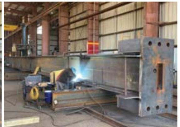
Precision Build (PB) recently began fabrication work on 14 million pounds of heavy steel columns. A fast-to-the-hook schedule requires coordination between the subcontractor, vendors, and our customer for this project to be successful. To support all other operations, detailed logistics for the project are critical, with up to 20 loads of material coming in or out of the facility each day.
