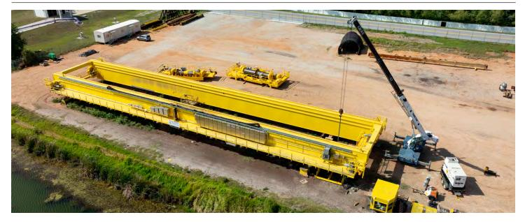
PB has successfully completed fabrication, assembly, and coatings on two massive overhead crane systems for a valued customer. These cranes were custom-made to meet the highest standards of quality, safety and performance based on our customer's design. They measure 12' in height, 30' in width, 195' in length, and can lift up to 120 tons each. The cranes are designed to handle heavy-duty industrial
